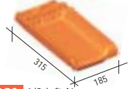
891 RS 1/2 left Norman verge (no overlap) - 4 per m. - 2 kg.
